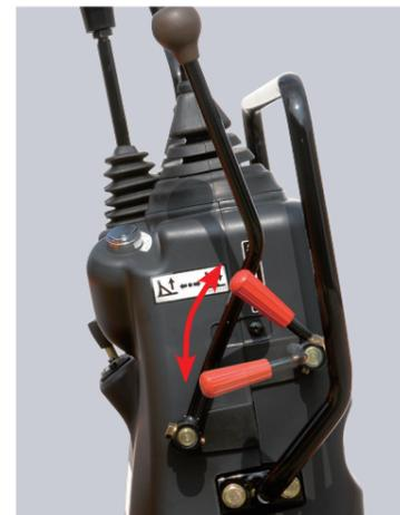
**Lock Lever Allows Lock/Neutral Engine Starting**
